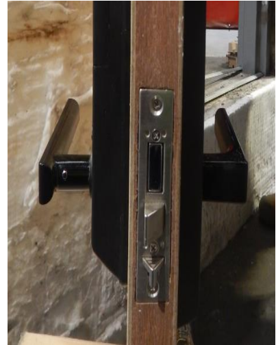
Figure 3 Latch edge of the tested hardware
